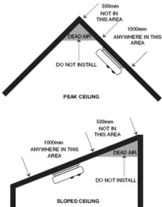
Smoke alarm should be located between 500 and 1500mm from the highest point.
